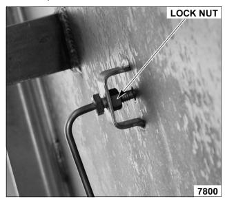
Reverse procedure to install and check braising pan for proper operation. **NOTE:** When installing: Route thermocouple wire in the same manner thru the metal clamps on the hinge & frame. Tighten thermocouple just until it touches the pan; do not over tighten or damage to the thermocouple may occur.
